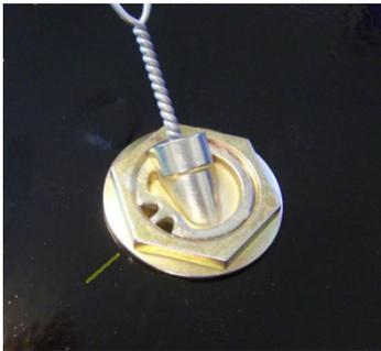
6. Insert the galley brush into the oil level gauge adapter and into the oil pan. **Insert it all the way so the bristles are all in the oil pan.** This will prevent the adapter from falling into the oil pan. Tie a heavy string to the open end of the brush in case it is dropped into the oil pan for quick retrieval.
