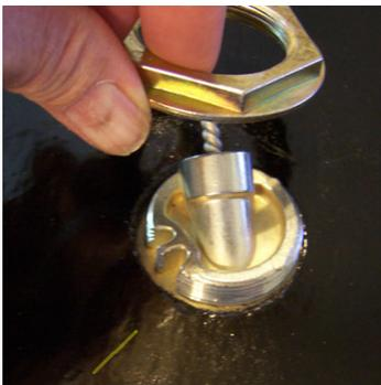
7. Remove the adapter retainer nut and discard the nut.
