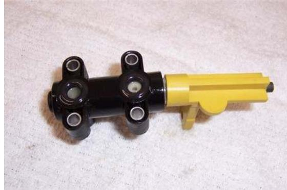
9. Lubricate the new main sealing o-rings with clean diesel fuel and press them into the valve with your thumb. Place the lever back on the valve and rotate the valve so you can see the opening in both the top and bottom o-rings. Note that the lever should be facing towards the rear of the valve in the position shown here. It will be important that you maintain this orientation when the valve is re-installed.
