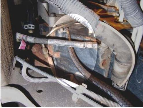
1. Locate the drain tube that comes from the fuel bowl. It is under the passenger side valve cover, directly below the A/C compressor. Slide a 30" piece of hose over the tube and route it to the shop floor. You should place a catch can under the hose so when the fuel bowl is drained, the fuel will be contained in the catch can.
