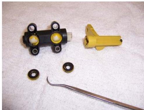
6. Once you have removed the drain valve, use a pick tool to remove the old o-rings.
