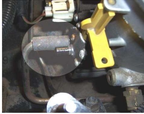
4. Shut the fuel valve off once the bowl has drained. Pull the drain tube connector off of the valve. The nipple that the hose connects to is plastic so be careful not to force it up or down, just pull straight towards the rear of the block. There are four screws holding the valve assembly to the bowl. (pre-99 OBS 7.3L have only 2 screws)
