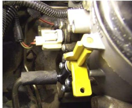
10. Place the valve against the rear of the fuel bowl so that the lever fits into the guide hole of the fuel bowl. Install the four screws and tighten them to 5-8 Lb-in. Re-attach the fuel drain tube to the drain valve's plastic nipple.
