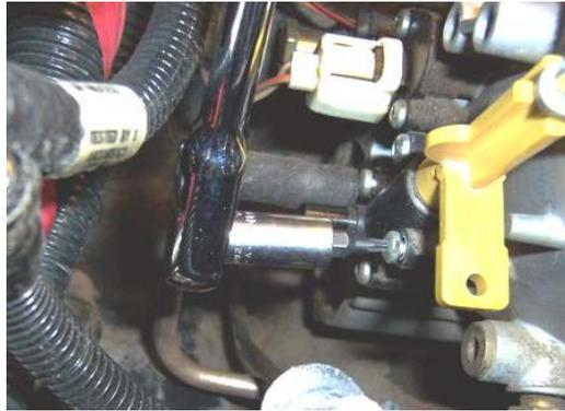
5. The screws require a #20 torx bit. Using a 1/4" ratchet and socket to hold the torx bit, remove all four screws. It will be helpful to keep a magnetic pick up tool or grab tool handy in case you drop your wrench in the engine block valley.
