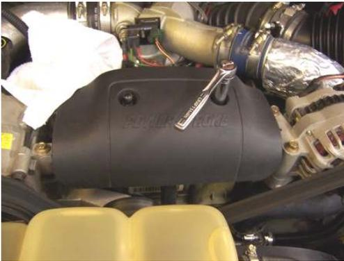
2. Remove the engine cover to gain better access to the fuel bowl. The black nut caps that hold the cover require a 13mm deep socket. If your caps are missing, the nuts are 12mm.
