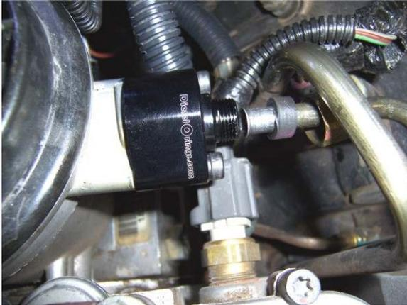
**⚠ IMPORTANT:** If replacing the cap due to breakage of the factory cap and you cut and re-flared the return line, the flare **MUST** be small enough so the flare fits inside the threaded nipple on the regulator cap. If the flare is too large, the compression sleeve will not seal the line to the housing.
