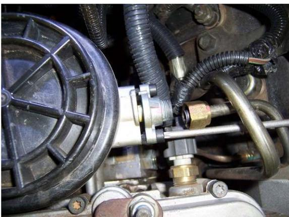
3. With a #25 torx screwdriver or bit, remove the 2 bolts from the FPR cap evenly. If you remove one completely and then the other, the pressure from the spring can put undue strain on the bolt ear of the remaining bolt. Pull the cap straight off the spring and remove it from the brass regulator piston seat.
