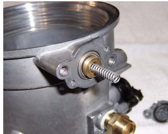
12. Tighten the new, longer FPR bolts evenly and do not allow the cap to twist sideways when attempting to start threading the new bolts to the fuel bowl.
